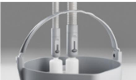
10. Connect suction hoses to Pulse Cleaner – adaptors may be required as hose sizes vary. Pulsed aspiration of the solution will happen automatically.
